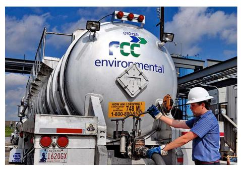
Operator at the New Orleans plant unloading a truck that collects used engine oil.
